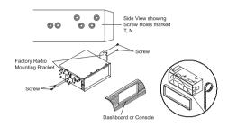
Fasten the unit to the factory radio mounting brackets. Align the screw holes on the bracket with the screw holes on the unit, and then tighten the screws (5x5mm) on each side.
